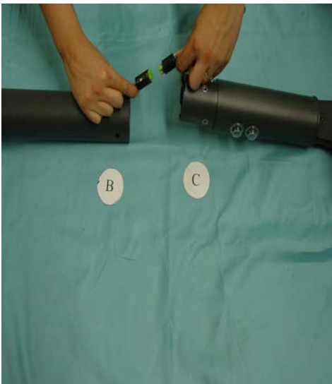
6. Connect the top part of the 993 with the two heaters. Connect the 2 connectors, run in the cable and insert pole B in pole C. Tighten the 4 6MA socket head screws, positioning and then tightening them. At this point the heater is ready for use.
